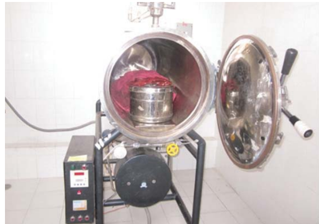
Figure 3. Autoclave used for treatment of infectious waste
