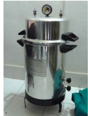
The day care centre's waste is disinfected in a 40-litre autoclave. Most of the electricity comes from solar power system (see separate case study)
